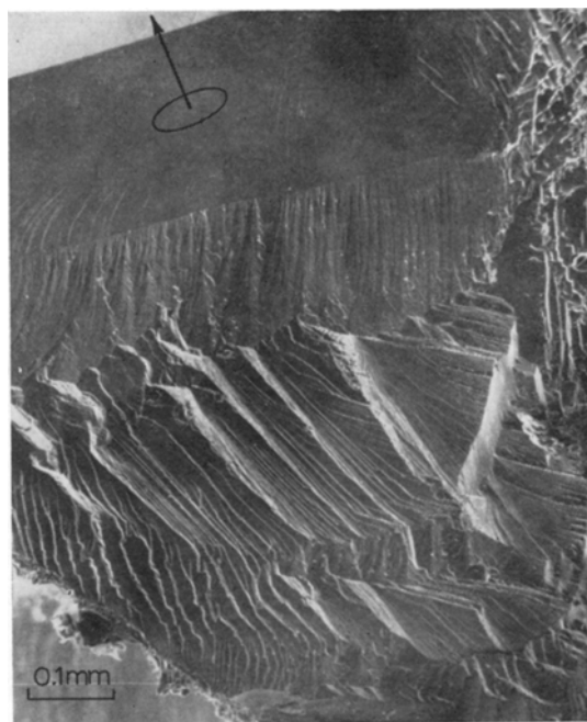
Figure 2 Scanning electron micrograph of Ti-Mo crystalline wire sample fractured partially across a grain-boundary. The grain-boundary plane is observed on the extremely smooth area. The arrow indicates the normal to the boundary, coincident with [111] and the wire axis.
